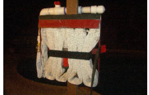
...as the hose bundle is secured at Box upper flap with velcro release strap hidden on reverse.
